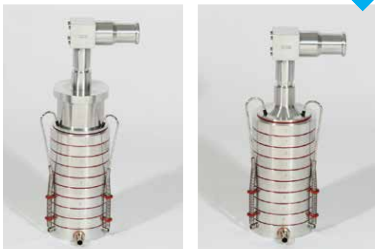
Figure 2: The modified induction port specified for APSD measurement necessitates the use of a modified ACI pre-separator for inhalation powders (left) and a modified ACI inlet cone for inhalation aerosols (right)
