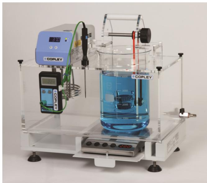
**Figure 6:** Disintegration testing apparatus for hydrophilic suppositories can also be used to measure the softening times of lipophilic products.
