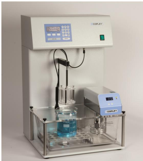
**Figure 2:** A simple apparatus for standardised, reproducible disintegration testing
