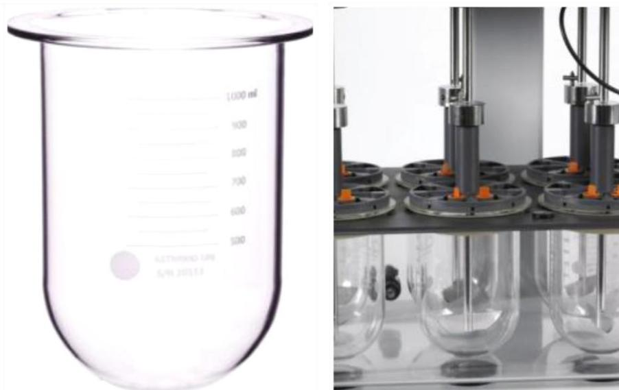
**Figure 2: The vacuum formed EMC Dissolution Vessel and EMC Test Station (Copley Scientific)**
