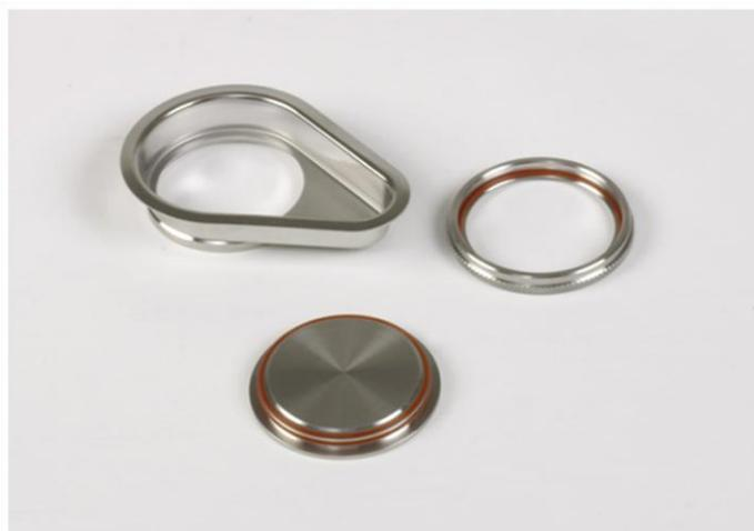
**Figure 3: NGI dissolution cup and membrane holder (Copley Scientific, UK)**
