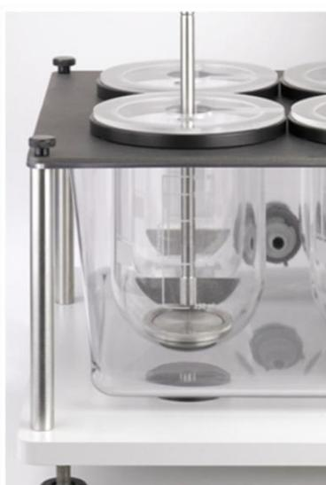
**Figure 4: NGI membrane holder in position in the vessel of a standard USP Apparatus 2**
