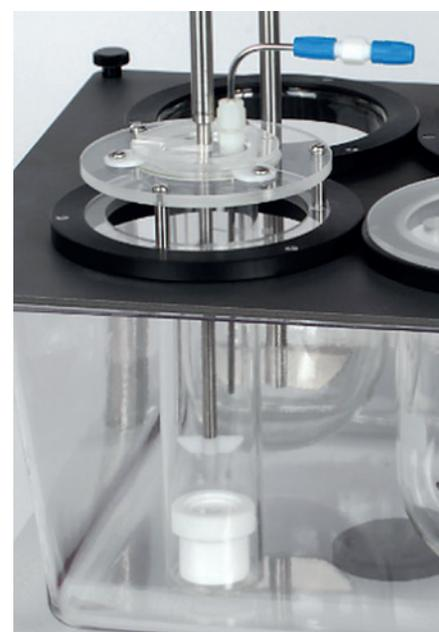
Figure 5: An immersion cell (above) is used with the conventional USP Apparatus 2 fitted with a small volume conversion kit, as shown on the right.
