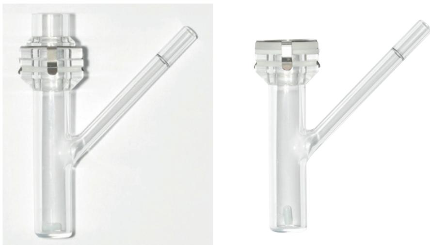
Figure 2: A Model B VDC in an open (left) and closed (right) configuration.
