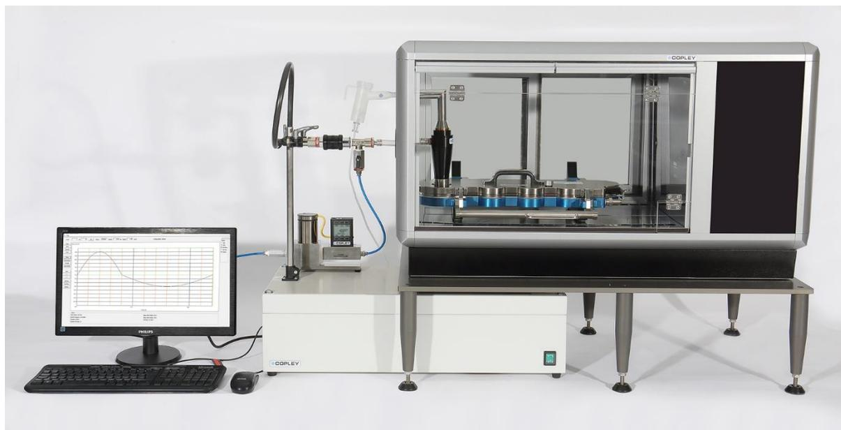
**Copley Scientific's efficient, integrated solution for measuring clinically representative APSD data for nebulisers, complete with twin-port NGI Cooler, NGI Cooler Stand and automated compressed air flow control.**
