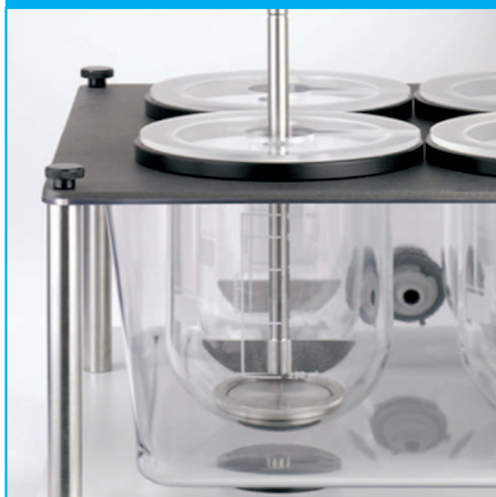
Figure 2: NGI membrane holder in position in the vessel of a standard USP Method 2 test apparatus.
