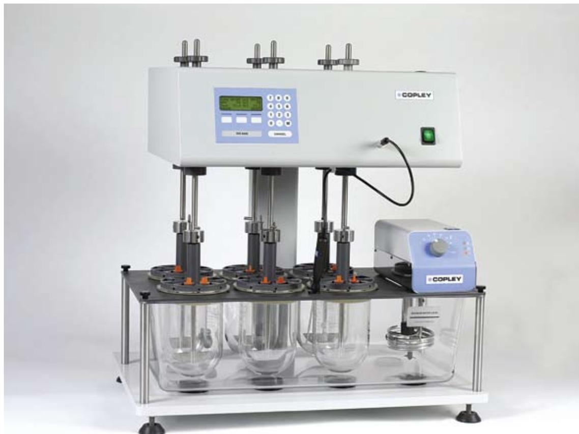
**Figure 1:** A modern-day dissolution tester (Copley DIS-EMC 6000) with enhanced mechanical calibration features.
