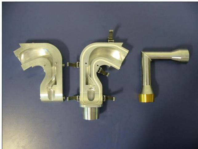
**Figure 3:** The AIT has a more human-like geometry than the USP/Ph.Eur. induction port but is easily manufactured to very close tolerances for consistent analysis
