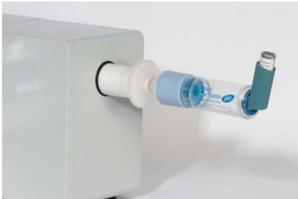
Figure 6: Using a breathing simulator to test a pMDI with spacer
