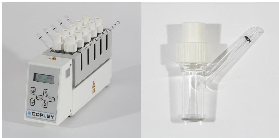
**CAPTION: The HDT 1000 Vertical Diffusion Cell Test System (left) pictured with the new skin specific VDCs (right).**
