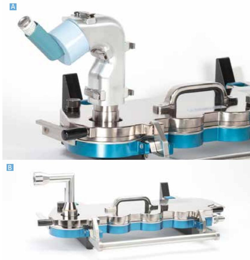
**Figure 4:** Idealised throat models (A) more accurately reflects the amount of drug captured in the throat than a standard USP/Ph Eur induction port (B)
