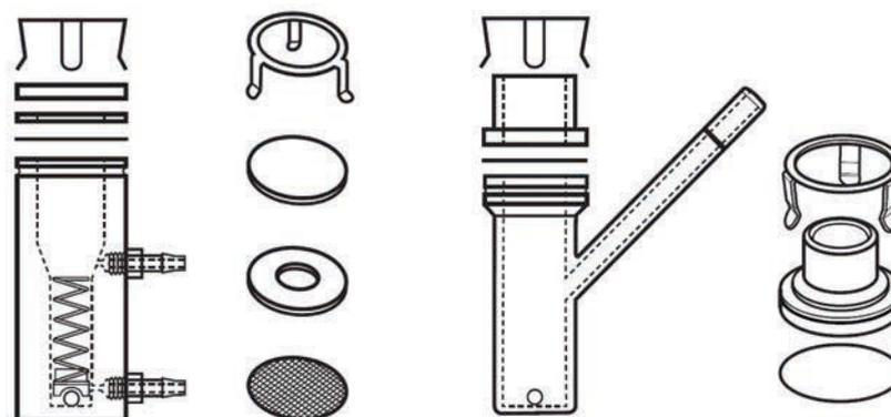
Figure 1: Line Drawings showing the construction of the VDCs described in USP <1724> as Model A (left) and Models B and C (right)
