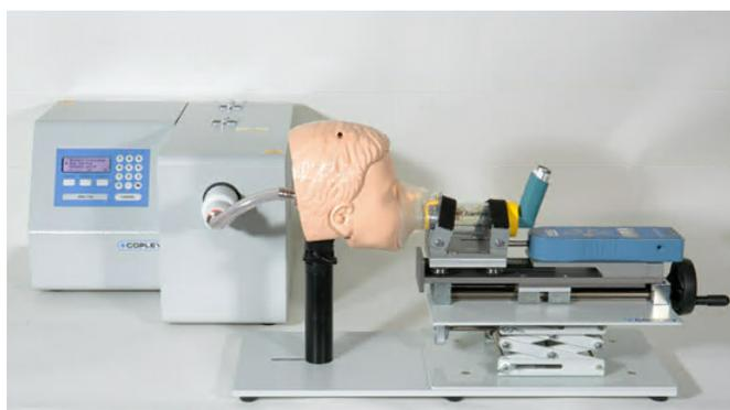
**Figure 6:** Newly introduced test methods for MDIs with spacers and VHCs specify the use of realistic face models when testing the face masks used with these add-on devices.
