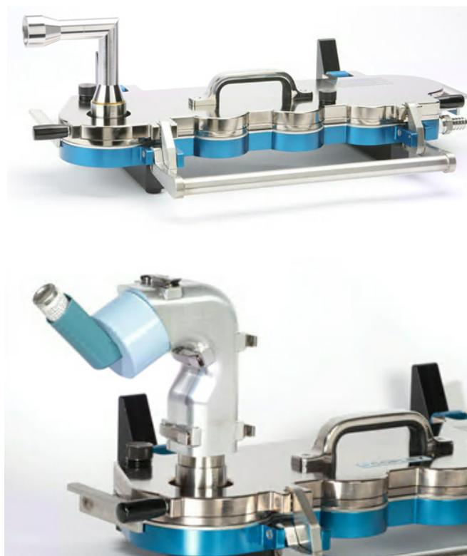
**Figure 4:** Use of an Alberta Idealised Throat (AIT) (bottom) more accurately reflects the amount of drug captured in the throat than a standard USP/Ph.Eur. induction port (top).
