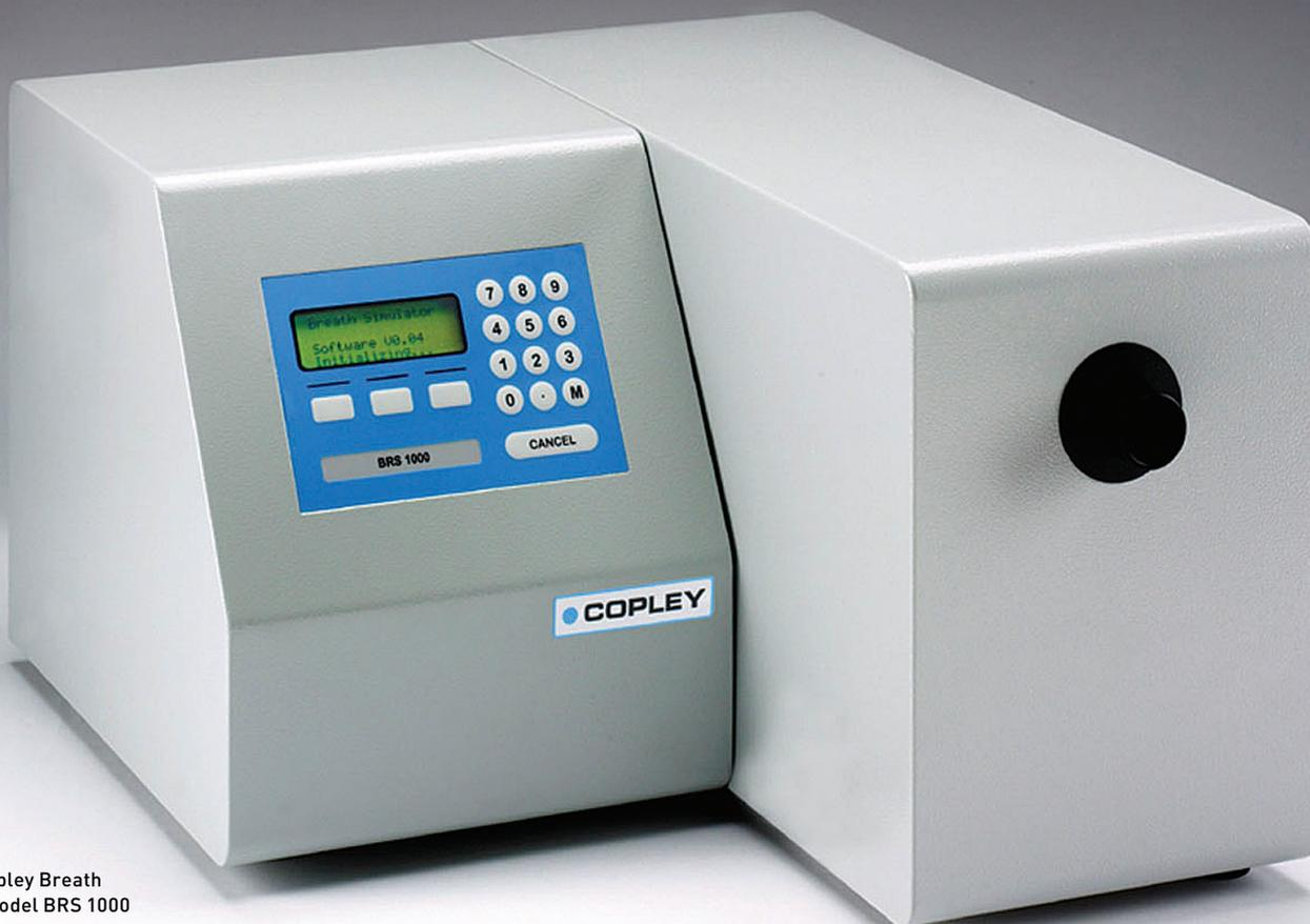
Figure 1: Copley Breath Simulator Model BRS 1000
