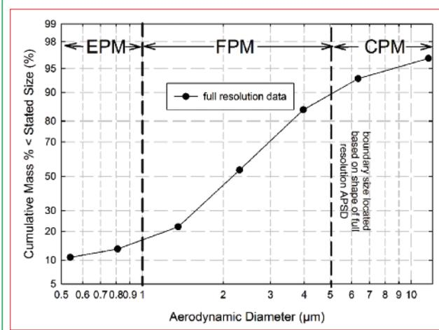
ratus includes the induction port and pre-separator, summing the FPM and CPM gives the mass that actually enters the abbreviated impactor.
