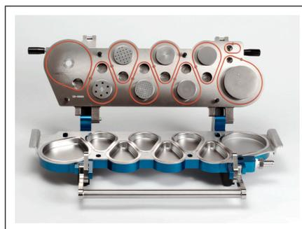
*The NGI has calibrated performance at 15 L/min and high capacity collection cups making it particularly suitable for the characterisation of nebulisers.*
