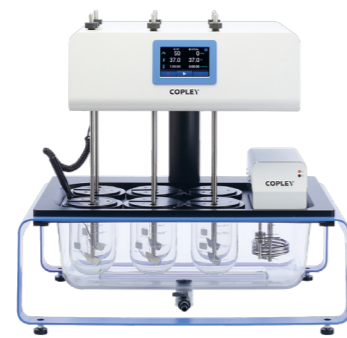
Figure 2: The DIS 600i with six stations
