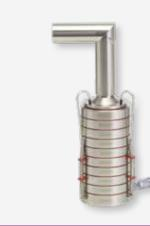
If the spacer/VHC is intended for adults, then the standard ACI or NGI should be used with a suitable vacuum pump capable of producing 28.3 or 30 L/min respectively. If the add-on device is intended for neonates, infants or small children, then only the NGI should be used as this can be used at the lower flow rate of 15 L/min.
