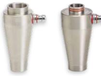
Our Mixing Inlets are designed to allow the cascade impactor to operate at a constant flow rate, whilst permitting a lower fixed or variable rate to pass through the inhaler. Positioned between the induction port/ throat/nasal inlet and cascade impactor, Mixing Inlets decouple the flow rate through the device from the air flow drawn through the impactor, enabling more representative testing.
