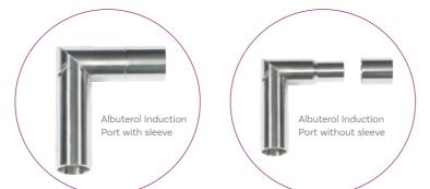
APSD measurement is conducted using a standard ACI equipped with a specially modified induction port. A special Inlet Sleeve is available that slips over the induction port inlet, to enable the induction port to be used with regular mouthpiece adapters used on USP/NGI induction ports.
