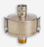
In most cases, the MOC eliminates the need for a final paper filter, having an 80% collection efficiency of 0.3 micron particles at 30 L/min. If ultra-fine particles are present and at flow rates below 30 L/min, then an internal or external filter
