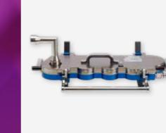
The test set-up is shown with an NGI but an ACI is equally suitable for the assessment of nasal powders. The Fast Screening Andersen (FSA) impactor is a reduced stack plus filter version of the ACI. As little deposition is expected in the lower stages, the FSA may be used to assess the APSD characteristics of nasal powders.
