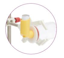
The apparatus uses a solid plastic firing adapter, instead of a mouthpiece adapter, to accept an inhaler with a circular mouthpiece of corresponding dimensions. Alternatively, a silicone Mouthpiece Adapter (page 203) can also be used.
