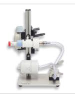
Ideal for maximising the aerolisation of nasal drug products in the assessment of fine particles by cascade impaction, Glass Expansion Chambers are available for a wide range of nasal drug product applications.
