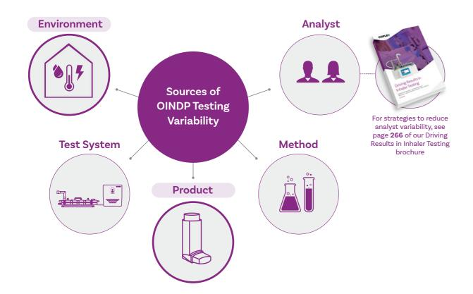
Localised changes in laboratory temperature and humidity, and also the presence of electrostatic charge, are known to have a direct influence on the dose emission and aerosol generation performance of OINDPs, thereby compromising DDU and APSD test data integrity.
