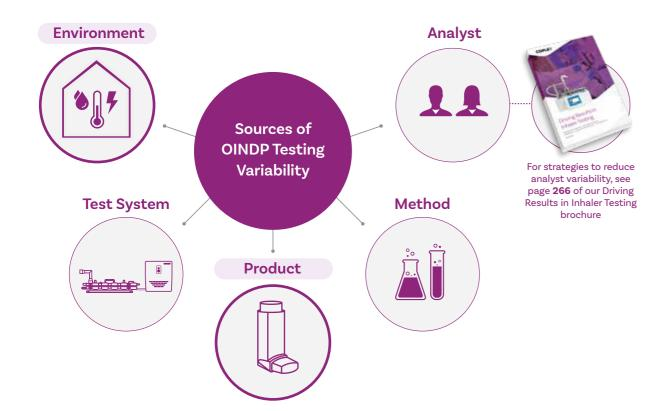
Localised changes in laboratory temperature and humidity, and also the presence of electrostatic charge, are known to have a direct influence on the dose emission and aerosol generation performance of OINDPs, thereby compromising DDU and APSD test data integrity.
