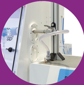
EnviroMate with Breathing Simulator BRS 200i for nebuliser testing
