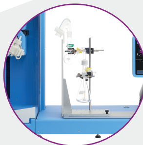
Glass Twin Impinger with Nasal Adapter
