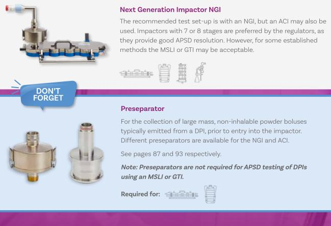
In addition to the above, the following is needed to complete a fully-operational test set-up for the APSD measurement of DPIs:
