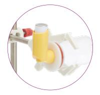
The original apparatus used a solid plastic firing adapter, instead of a mouthpiece adapter, to accept an inhaler with a circular mouthpiece of corresponding dimensions. Alternatively, a silicone Mouthpiece Adapter (page 211) could be used.
