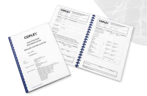
According to USP Chapter <1058>, Analytical Instrument Qualification is "the collection of documented evidence that an instrument performs suitably for its intended purpose".
