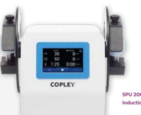
SPU 200i fitted with 2 x ACI Induction Ports
