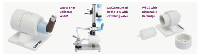
The Waste Shot Collector WSC2 is a compact vacuum filtration system suitable for use with a range of devices. It can be used in either standalone mode or integrated into the Inhaler Testing Workstation<sup>™</sup> ITW (see page 204), via a switching valve, whereby the vacuum pump used for the DUSA powers both sampling and waste collection units.
