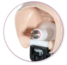
Filter Holder and Adapter located in a cavity behind the face model's lips
