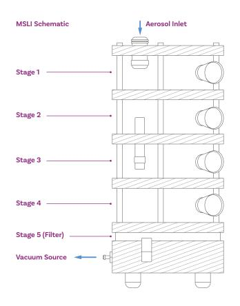
The aerosol stream is drawn into the top of the MSLI, passing first through Stage 1 which acts as a preseparator. Particles with sufficient inertia will impact on the moist surface of the sintered glass disc. Those with insufficient inertia will pass through to Stage 2. The same process of impaction and particle selection takes place until the final filter stage (Stage 5), which captures any remaining fine particles.
