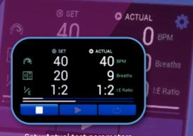
Set v Actual test parameters (during test run, with test progress bar and enhanced visualisation of breath status)
