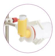
The original apparatus used a solid plastic firing adapter, instead of a mouthpiece adapter, to accept an inhaler with a circular mouthpiece of corresponding dimensions. Alternatively, a silicone Mouthpiece Adapter (page 211) could be used.
