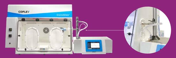
EnviroMate with Breathing Simulator BRS 200i for nebuliser testing
