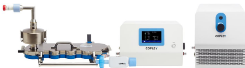
Figure 1A – a classic test setup for APSD measurement for DPIs with NGI, standard USP/Ph.Eur. induction port, flow meter, critical flow controller, and vacuum pump
