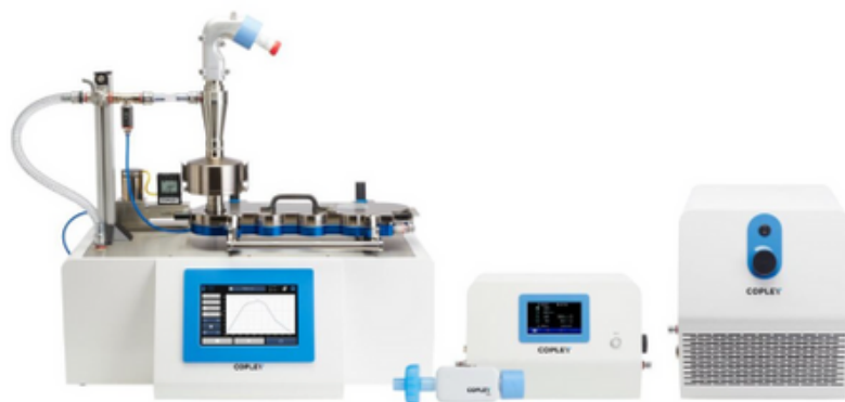
Figure 1B – a comparable test setup for realistic APSD measurement additionally incorporating breathing simulator and mixing inlet, with an Alberta Idealized Throat in place of the standard induction port
