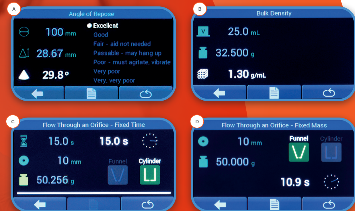
A: Angle of Repose B: Bulk Density C: Flow Through an Orifice via Cylinder - Fixed Time Density D: Flow Through an Orifice via Funnel - Fixed Mass
